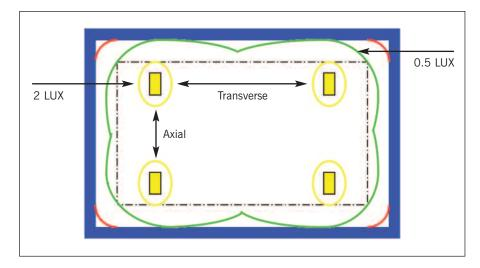
Fig 8 - Mounting positions for open area lighting
